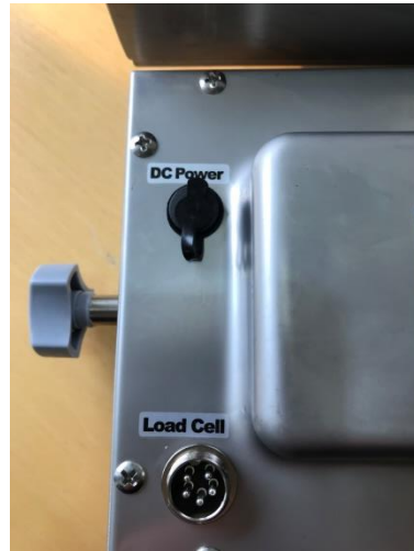
Power supply port & Load Cell (Weigher) port
